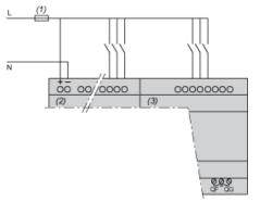
(1) 1 A quick-blow fuse or circuit-breaker. NOTE: QF and QG: 5 A for SR3XT141•• SR3B261FU
